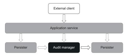
Figure 6.15 ApplicationService glues the functional core (AuditManager) and the mutable shell (Persister) together and provides an entry point for external clients. In the hexagonal architecture taxonomy, ApplicationService and Persister are part of the application services layer, while AuditManager belongs to the domain model.
