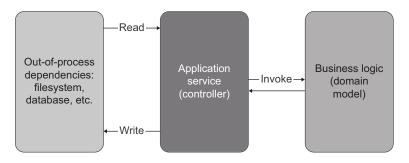
Figure 7.10 Hexagonal and functional architectures work best when all references to out-of-process dependencies can be pushed to the edges of business operations.
