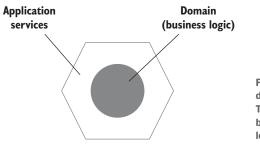
Figure 5.8 A typical application consists of a domain layer and an application services layer. The domain layer contains the application's business logic; application services tie that logic to business use cases.
